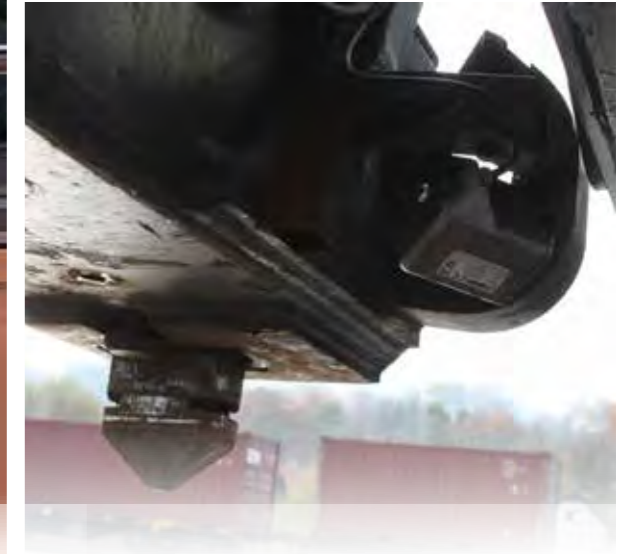
The cameras are mounted in such a way as to provide an optimum view onto the twistlocks.
