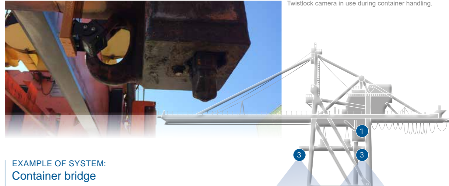
Twistlock camera in use during container handling.
