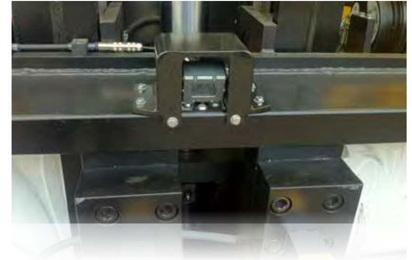
A carriage mounted camera is lifted simultaneously with the load.
