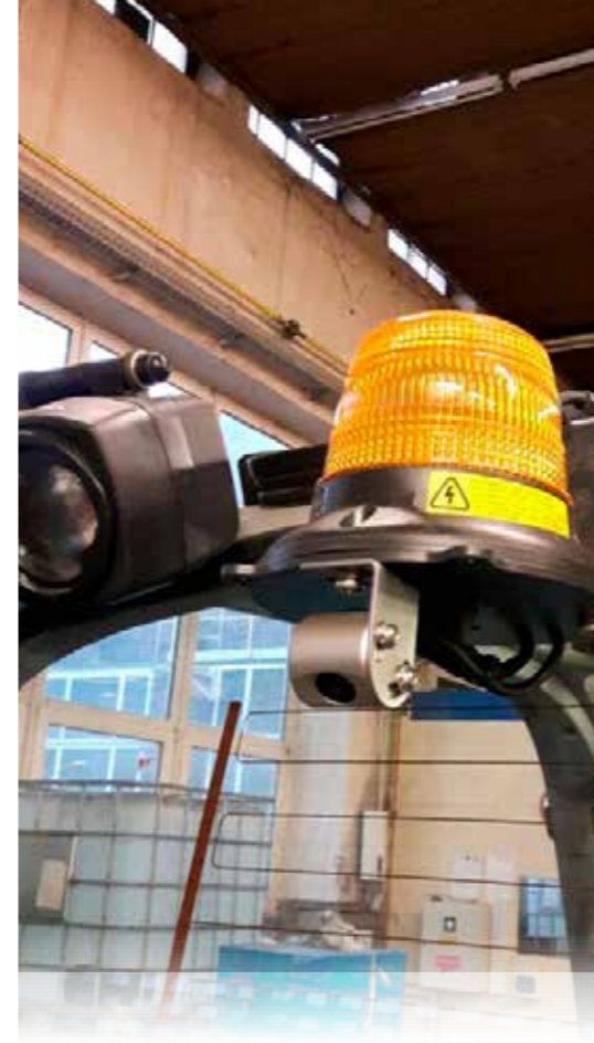
Various mounting positions for back room monitoring
