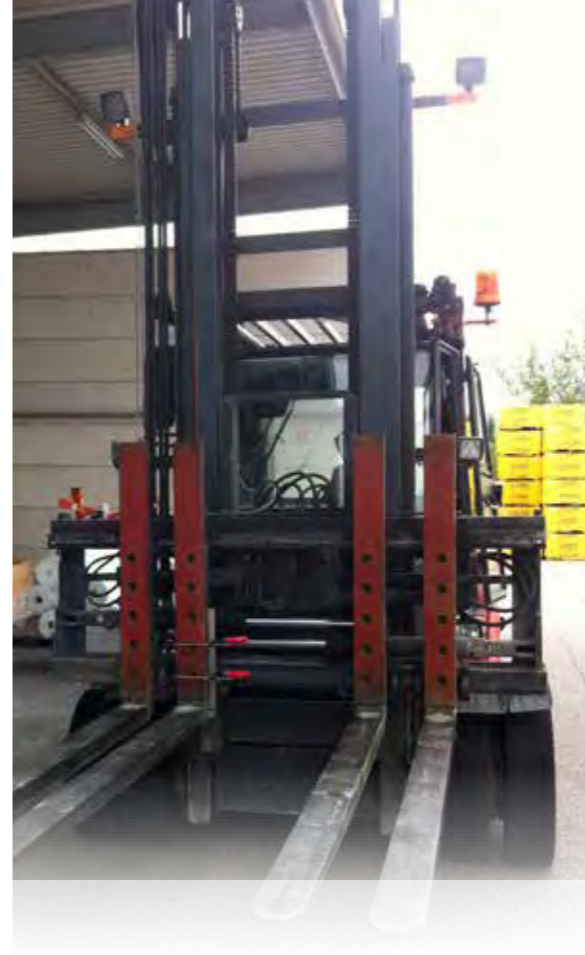
A carriage mounted camera is lifted simultaneously with the load.
