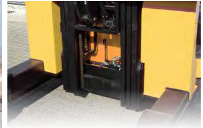
Motec mast or fork carrier camera – always level with the load.
