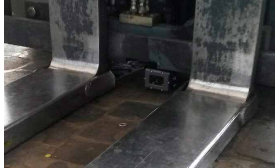
MVS system: MC3000B as optional fork carrier camera. Wide-angle camera MC7180N for lateral and rear view monitoring.
