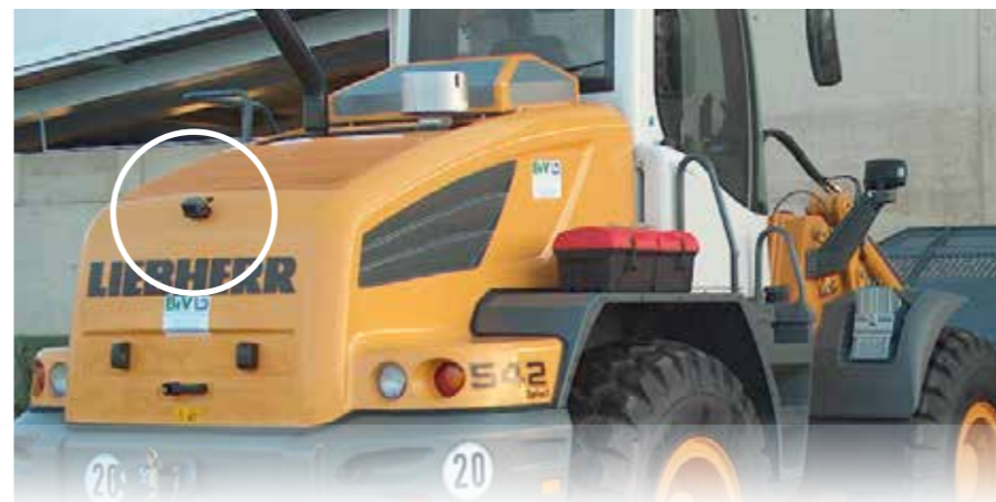
Front-end loader with MC3000B heavy-duty monitor at the rear for rear-space monitoring.
