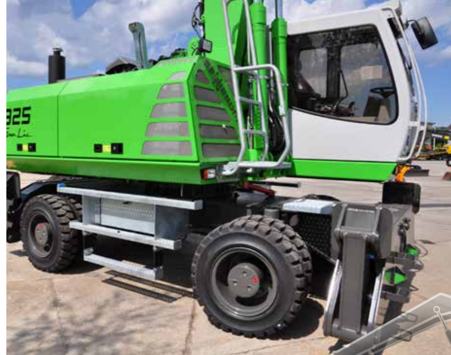
Mobile material handling excavator, fitted with a complete Motec camera and monitor system.
