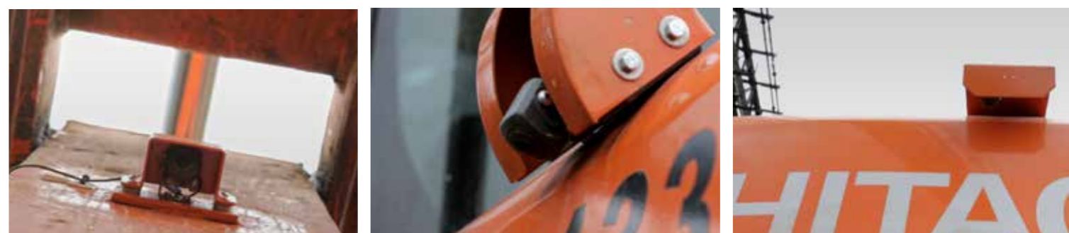
Left: Camera inside boom to monitor the working area Centre: Camera to monitor the vehicle's sides Right: Camera to monitor the vehicle's rear area
