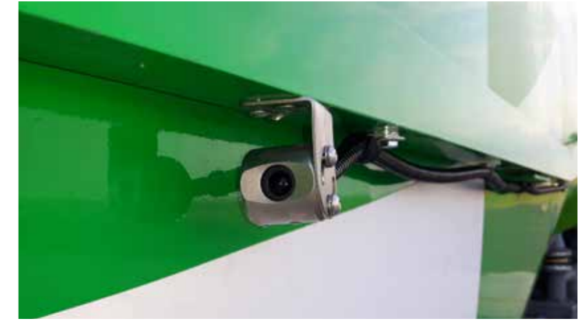
Mounting positions for the side camera.
