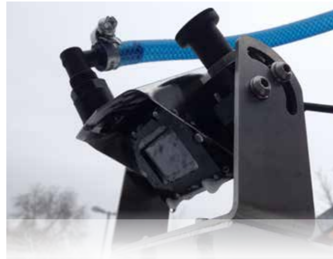
Side camera for monitoring the clearing blade (top left). Heavy duty rear view camera with cleaning system (bottom left).
