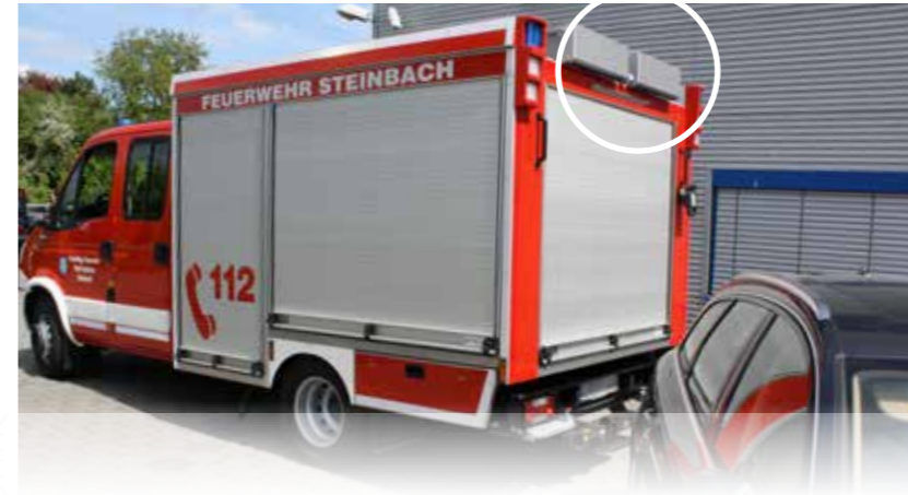
Heavy-duty camera for monitoring the rear area of the vehicle.
