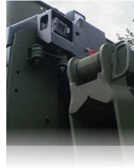
Heavy-duty camera on a recovery vehicle for supporting operation and monitoring of the underlift fork (left) and rear space monitoring (right).
