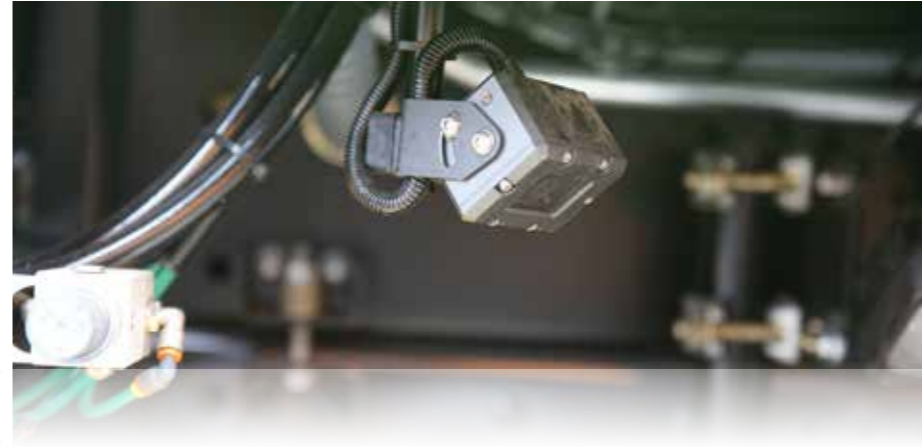
Using a camera to monitor the road sweeper's brushes.
