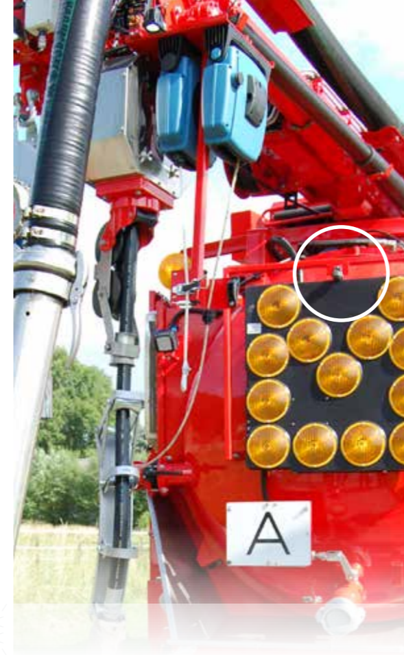
There are 4 cameras installed around the vehicle allow for a 360° birdseye view.
