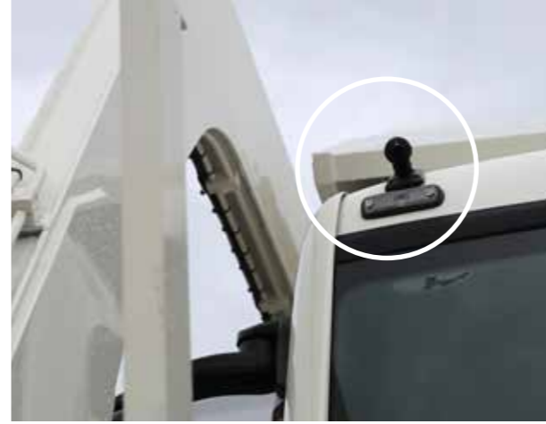
Refuse collection vehicles with camera for monitoring the front area of the vehicle. Heavy-duty camera for monitoring the rear and operating areas.
