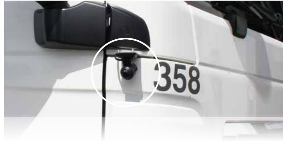
Tractor units with heavy-duty camera to increase the safety when making turns right.
